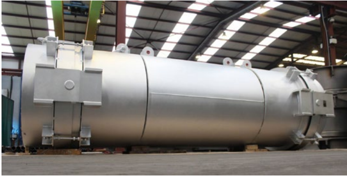
Double Gimbal - Hot Design - Floating Ring. Two ply monitored Inconel 625 LCF bellows. Design temperature: 760°C (flue gas) 538°C (bellows)
