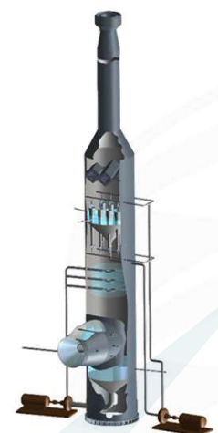
A single upflow tower controls many pollutants
