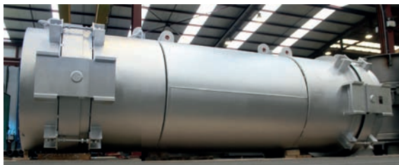
Double Gimbal – Hot Design - Floating Ring. Two ply monitored Inconel 625 LCF bellows. Design temperature: 760 °C (flue gas) 538 °C (bellows)
