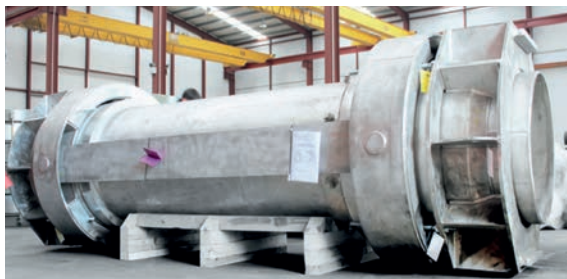
Universal – Cold wall design Two ply testable Inconel 625 LCF bellows. Design temperature: 768 °C (flue gas) 538 °C (bellows)
