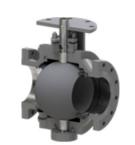
The MOGAS T-Series trunnion-mounted ball valve is available in both metalseated (3 to 36 inch) and soft-seated (3 to 60 inch) two- or three-piece designs, with operating temperature from -50° F to 400° F. The valve retains many of the time-tested features of the C-Series, such as an actuator mounting pad, but with a trunnion design. Its' reduced operating torque results in an overall less expensive valve and actuator package. (\* Not all size / pressure class combinations available.)
